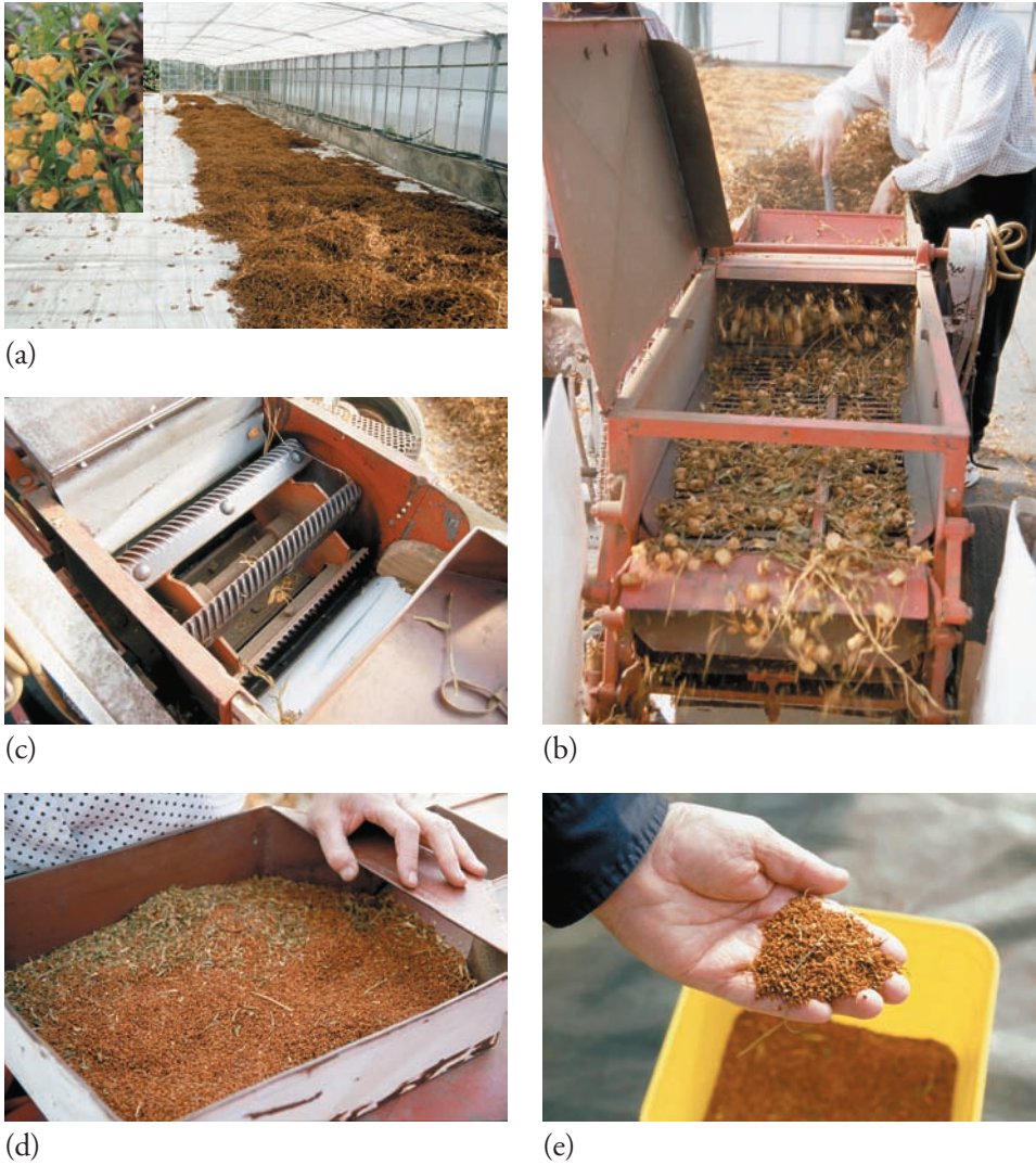
Figure 9 Sandersonia seed removal from a dry dehiscent capsule. (a) Hand-cut fruiting stems are cut and windrowed under protective cover for additional drying. (b) Pods are passed through a threshing machine to remove seeds. (c) The threshing cylinder with a rasp-bar is the most common thresher. (d and e) Proper threshing captures up to 90 percent of the available seeds, but additional conditioning is usually needed to remove fruit debris.
