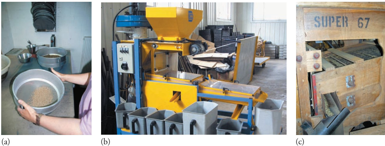
Figure 10 Seed conditioning based on seed size and shape. (a) Hand screens manually sift seeds from plant debris; (b) Mechanical cleaner and seed sizing units use aspiration (air movement) combined with screens of various shapes and sizes to remove seed debris and separate seeds into various size classes. (c) Close up of screens in a scalper unit that separates good seed from plant debris and other unwanted material.
