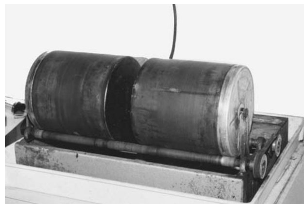
Figure 8 Seed scarifier used to abrade hard seeds with physical dormancy, such as legumes.
