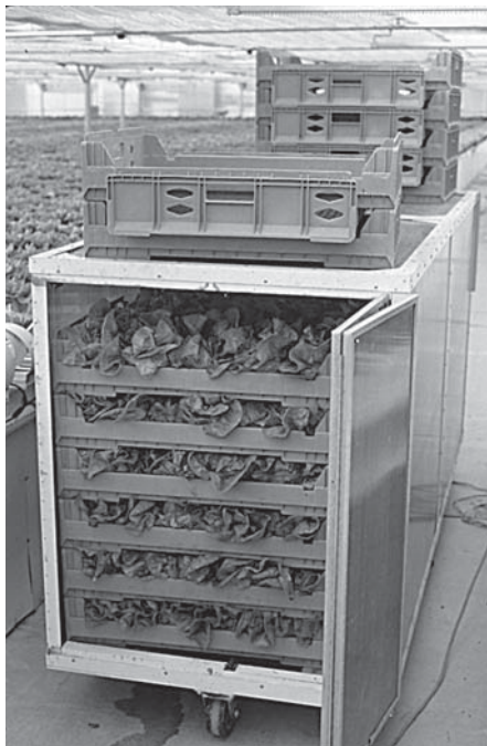
FIGURE 6.23 Mobile refrigeration unit with storage crates. (From F.W. Armstrong Ranch, Oak View, CA. With permission.)
