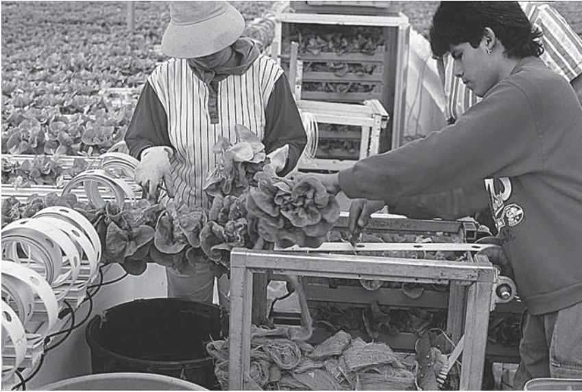
FIGURE 6.22 Use of harvesting–transplanting machine to pull rows of lettuce from the channels. Operators cut the lettuce off at their base as the tape passes to be rolled up below. (From F.W. Armstrong Ranch, Oak View, CA. With permission.)
