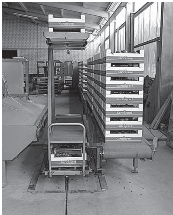
FIGURE 10.49 Tomatoes in cases are transferred to a belt to the packing area. (From FormFlex/Metazet Zwethove B.V., The Netherlands. With permission.)
