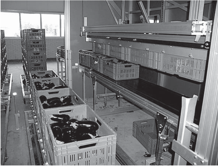
FIGURE 10.48 Eggplants in tote bins are automatically unloaded. (From FormFlex/Metazet Zwethove B.V., The Netherlands. With permission.)
