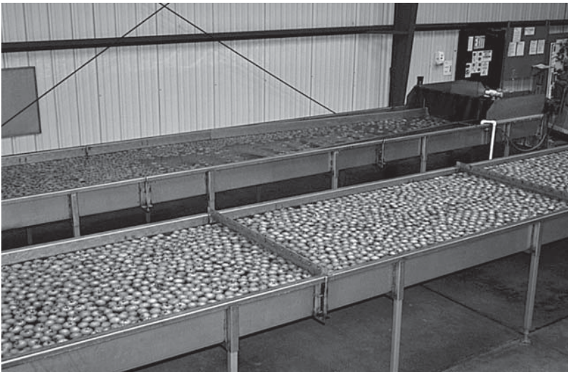
FIGURE 10.39 Tote bins with loose tomatoes are dumped into a water trough to float to the packing facility. (From Houweling Nurseries Oxnard, Inc., Camarillo, CA. With permission.)
