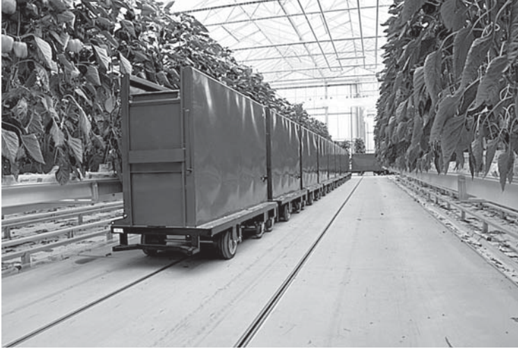
FIGURE 10.46 Bins for harvesting peppers and cucumbers travel on the chain track system. (From FormFlex/Metazet Zwethove B.V., The Netherlands. With permission.)
