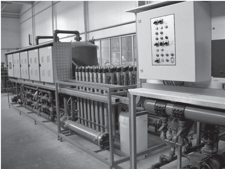
FIGURE 3.13 UV sterilization system for recirculation of nutrient solution. (From Bionatur Invernaderos Biologicos De Mexico, S.A. De C.V., Jocotitlan, Mexico. With permission.)
