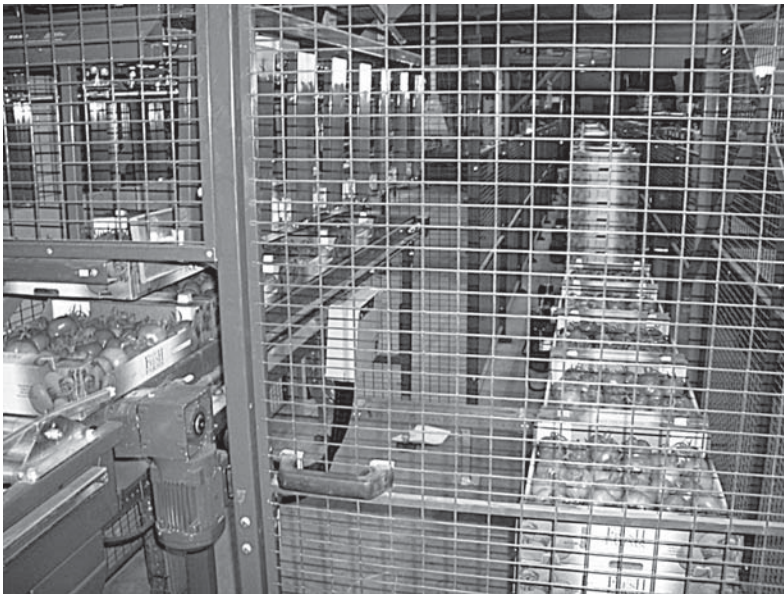
FIGURE 10.36 Machine lifts boxes from picking carts and places them on the grading–packing belt. (From Eurofresh Farms, Wilcox, AZ. With permission.)
