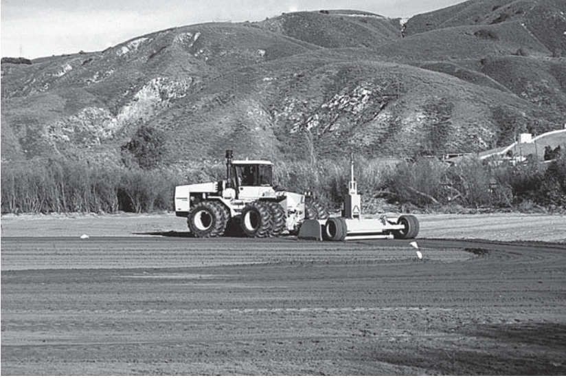
FIGURE 6.48 Laser leveling 3-acre field. (From California Watercress, Inc., Fillmore, CA. With permission.)
