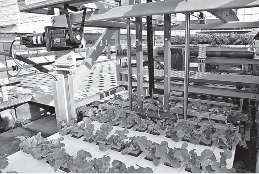
FIGURE 6.31 Plant robot transplanting to the NFT growing channels. (From Hortiplan, N.V., Belgium. With permission.)
