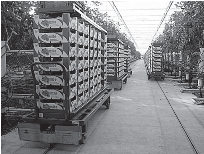
FIGURE 10.45 Carts moving in the central passageway on the chain track system. (From FormFlex/Metazet Zwethove B.V., The Netherlands. With permission.)
