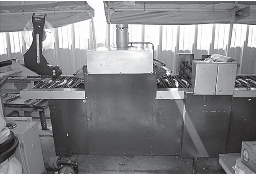
FIGURE 10.20 Large commercial shrink wrapping machine. (From Houweling Nurseries Oxnard, Inc., Camarillo, CA. With permission.)
