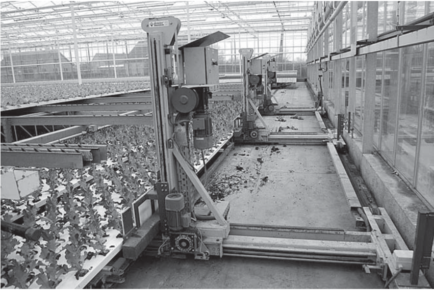
FIGURE 6.33 The gullies at the far end of the bench are lifted automatically to the top of the growing field (bench). (From Hortiplan, N.V., Belgium. With permission.)
